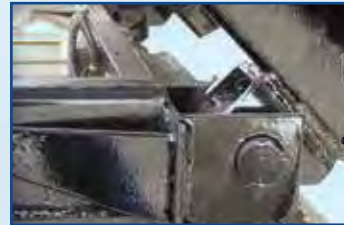
The Yardbird's heavy-duty platform hinge is greasable.
