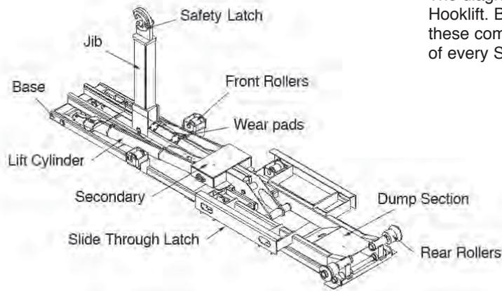
The diagram shows a typical Stellar Slider Hooklift. Below is a detailed explanation of these components which are an integral part of every Stellar Slider hydraulic Hooklift hoist.
