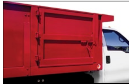
Doors open and lock to the side of the body with conveniently placed latches that can be operated from ground level.
