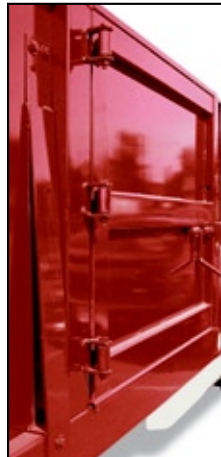
Side stiffener adds stability and strength to sides when cargo door swings open
