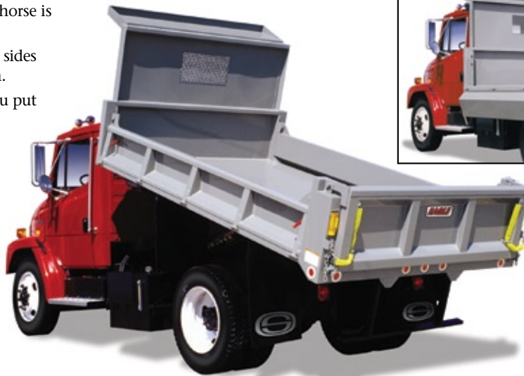
Two-piece drop sides with removable center post are standard on 14' and 16' models. 12' model has one-piece sides.
