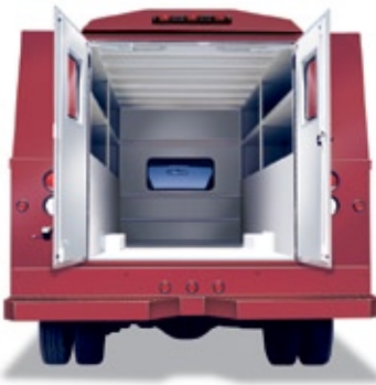
Compartment interiors and cargo area prime painted gray for enhanced illumination
